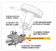
Loosen knurled screw 7, screw rotor 1 onto camera thread 13, tighten knurled screw 7 again. Fix the railing clamp to a suitable pipe with screw 12.
