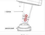
The rotor 1 can also be inserted directly into the QuickClamp.
